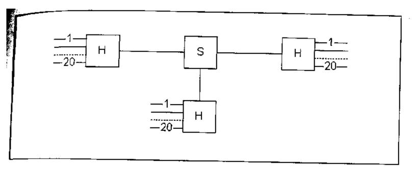
In the network above, assume that all the links are 100-Mbps links and that all the devices want to transmit at an average rate of R bps. Every hub is attached to the switch and to 20 devices. We assume that the traffic is symmetric: Each device sends at the same average rate to every other device. As we have done so far, we assume that the MAC protocol is perfectly efficient. What is the maximum possible value of R?
