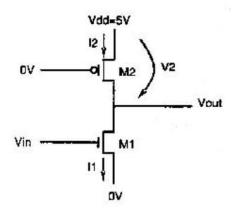
(a) [5 points] On the graph below, sketch carefully, I2 vs V2. Mark the regions of operation (i.e. off, triode, or saturation) and compute the transition points accurately (indicate voltage and current values in graph).
