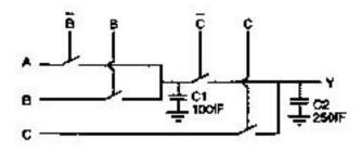
(a) [7 points] Write the truth table for the gate shown above with inputs A, B, and C, and output Y
