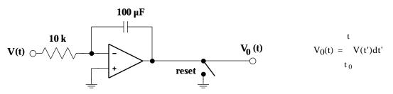
Set your circuit gains so that if the system is reset and subjected to a 0.1g acceleration for 1 s, the output is 50 mV.
