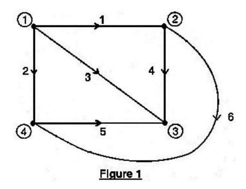
(a) Write down the reduced incidence matrix A with node 3 as the datum.
