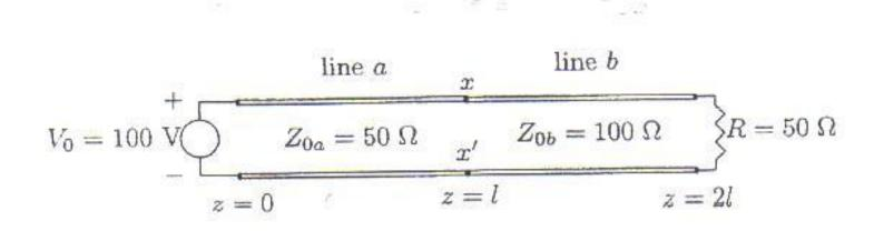
Two ideal lossless transmission lines, a and b, having lengths l = 200m and propagation velocities v = 2 E8 m/s, are connected together. The system is excited at the left on line a by an ideal dc voltage source  $V_0 = 100V$  and terminated at the right on line b by a resistor R = 50 ohms. Lines a and b have characteristic
