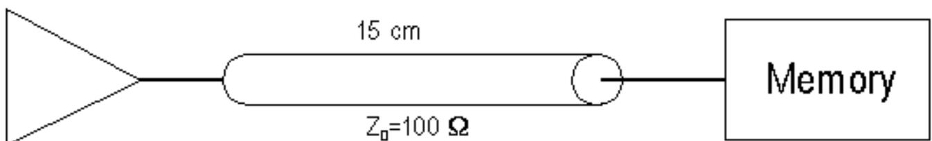
FIG. 4 Driving the memory through a transmission line
