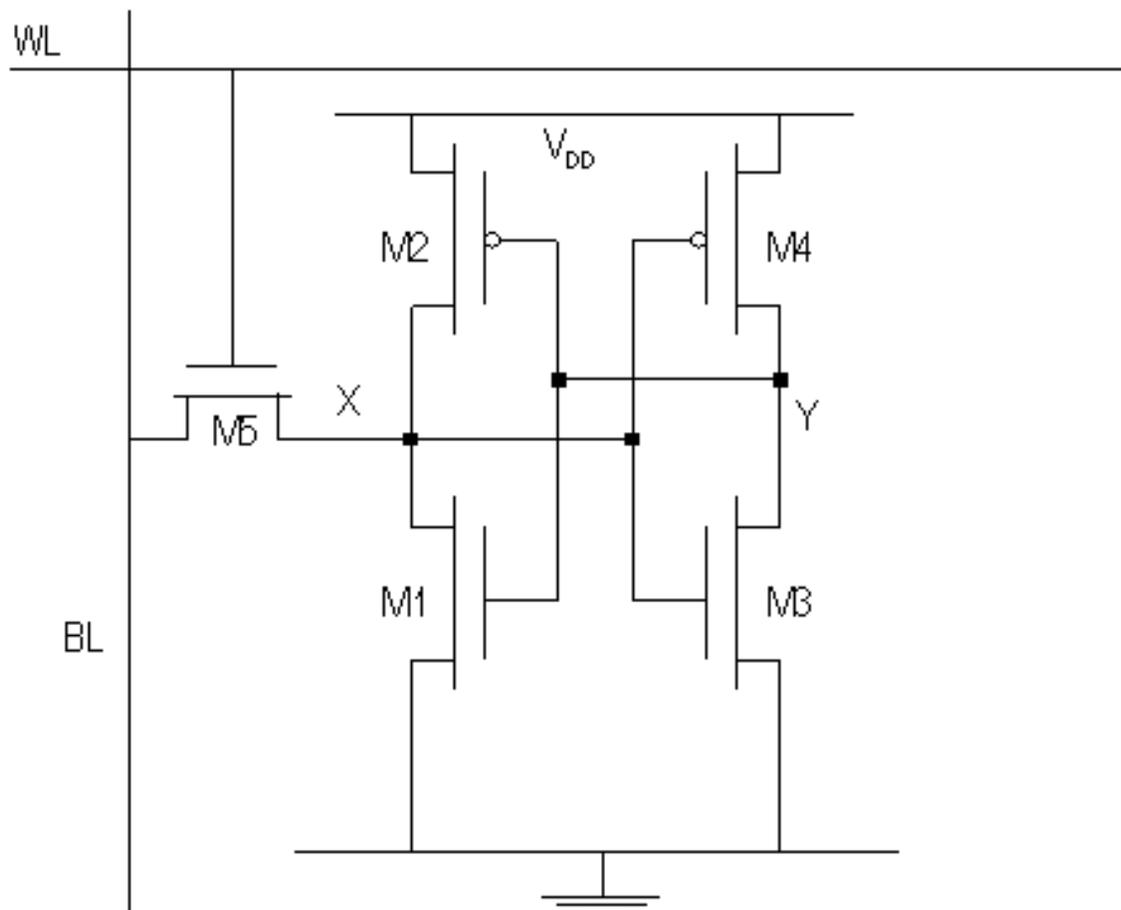
FIG. 1 5 transistor SRAM cell.
