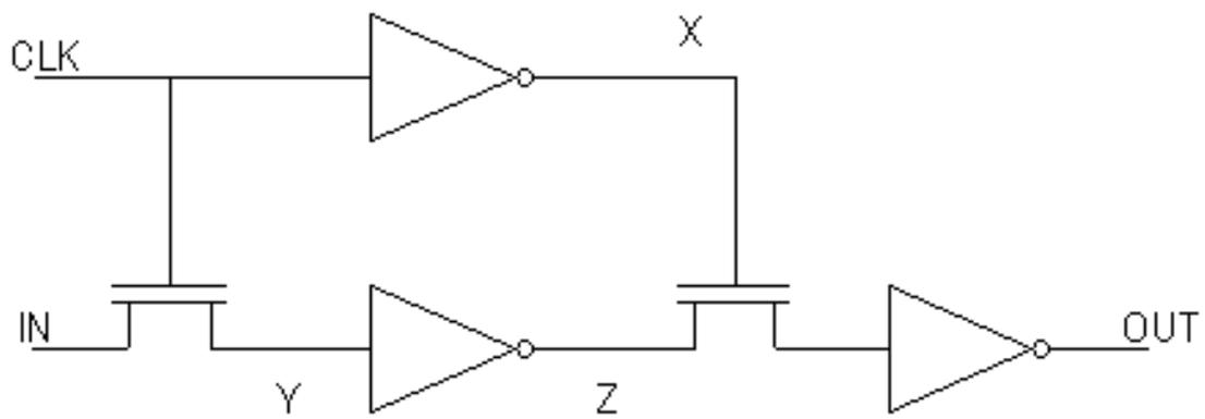
FIG. 5 Single clock register
