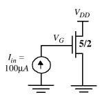
Consider the following simple circuit (implemented in the 1.2  $\mu$ m CMOS technology). Assume  $V_{DD}=3$  V and use the following transistor parameters:  $C_{ox}=1.75$  fF/ $\mu$ m<sup>2</sup>,  $x_j$  (lateral diffusion) = 0.15  $\mu$ m,  $C_{j0}=3.0\times10^{-4}$  F/m<sup>2</sup>,  $m_j=0.5$ ,  $C_{jsw}=8.0\times10^{-10}$  F/m,  $m_{jsw}=0.5$ .
