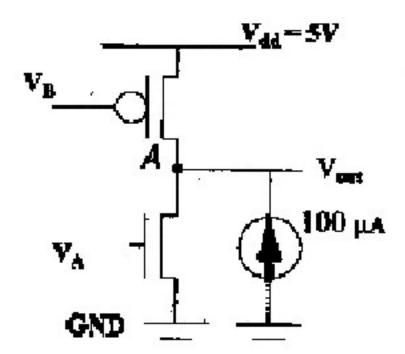
**1b**) (20 pts) Find the minimum value of (W/L)p such that when Va = 5V and Vb = 0V, the output voltage (including the 100 uA current) will be less than or equal to 1.5V. Note that both Va and Vb have changed from part a.
