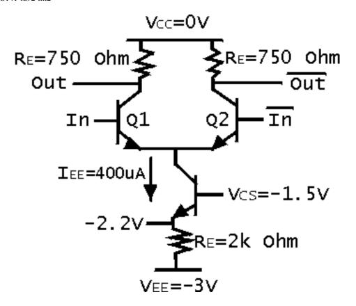
a). Determine the important points of the VTC ( $V_{OH}$ ,  $V_{OL}$ ,  $V_{IH}$ ,  $V_{IL}$  and  $V_{M}$ ). For the computation of  $V_{IH}$  and  $V_{IL}$ , you can use the simplified definition ( $V_{IL}$  is defined as the point where the transistor Q1 is carrying 1% of the current through the current source, while at  $V_{IH}$  transistor Q1 carries 99% of the total current).
