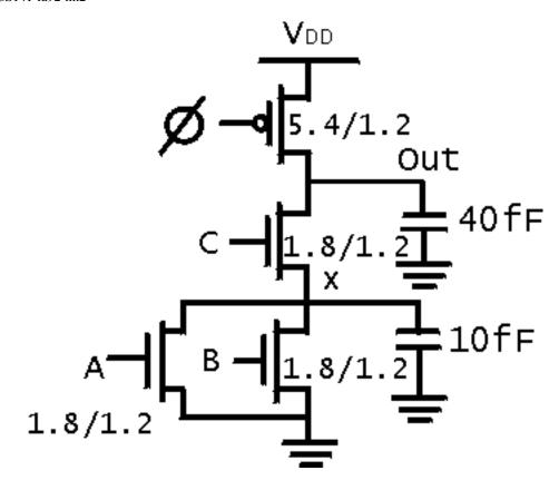
a). Is this circuit going to work under all conditions? If not, explain why and give a case when this circuit is not going to work.
