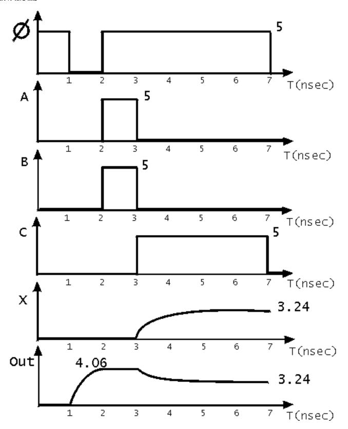
$t = 1 \text{ns} \rightarrow 2 \text{ns}$ : 40fF charging through PMOS at **Out**; no charge at **X** (floating) Vout =  $5(1 - \exp(-(t-1 \text{ns})/(15 \text{kOhm x } 40 \text{fF})))$  Vout(2 ns) =  $5(1 - \exp(-1 \text{ns}/0.6 \text{ns})) = 4.06$
