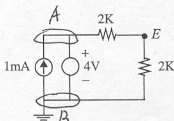
Voltage drop between A and B is determined by the Voltage Source.  $V_{AB} = 4V$
