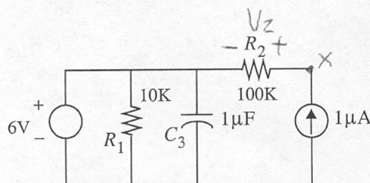
①  $V_z = iR = (1 \mu\text{A})(100K) = 1 \text{ V}$
