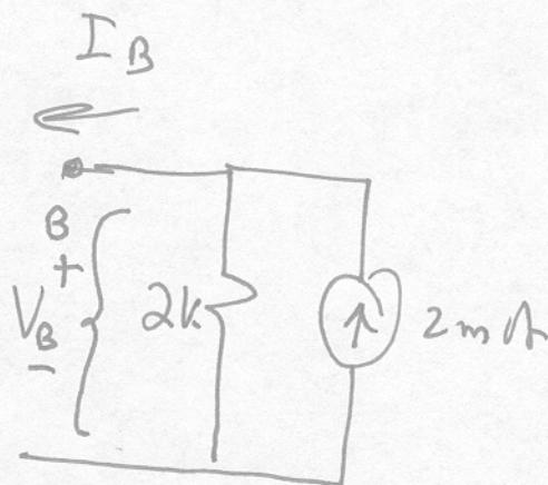
$I_B$  vs  $V_B$  is linear
