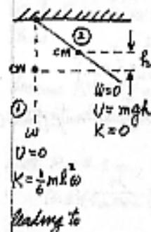
In the vertical position, the angular speed is  $\omega$ , the kinetic energy  $K = (\frac{1}{2})ml^2\omega^2$  and we define the gravitational potential energy  $U = 0$ .
