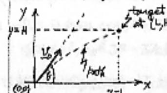
$$\begin{cases} x(t) = x_0 + (v_0 \cos \theta)t \\ y(t) = y_0 + (v_0 \sin \theta)t - \frac{1}{2}gt^2 \end{cases}$$
