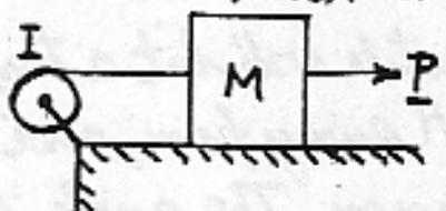
and is attached to a block of mass  $M$  which can slide over a frictionless horizontal surface. A horizontal force  $P$  is applied to the block. Calculate the magnitude  $a$  of the acceleration of the block.
