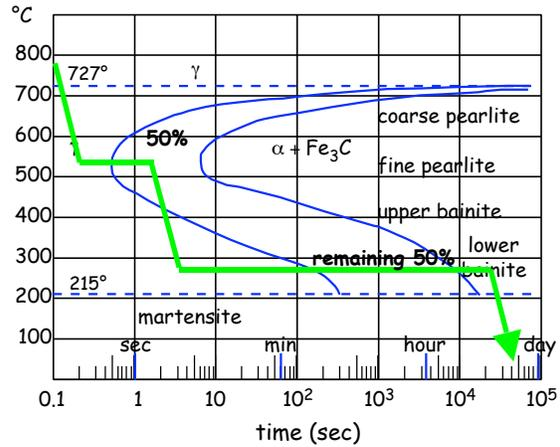
The only way this treatment can be an "interrupted quench" is to begin with the high temperature transformation (fine pearlite), holding isothermally until the reaction progresses half way between the start and finish lines. Note that this amounts to only a few seconds. The untransformed austenite is then lowered in temperature and held isothermally until it fully transforms to lower bainite as shown.
