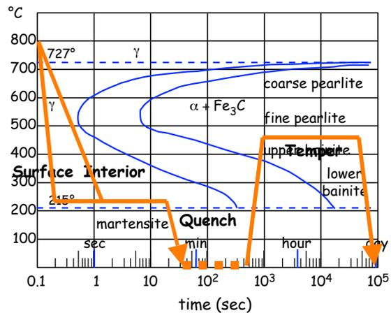
Both (a) and (b) are the classic, traditional methods used widely throughout the engineering community to prevent quench-cracking in large cross-section steel components.
