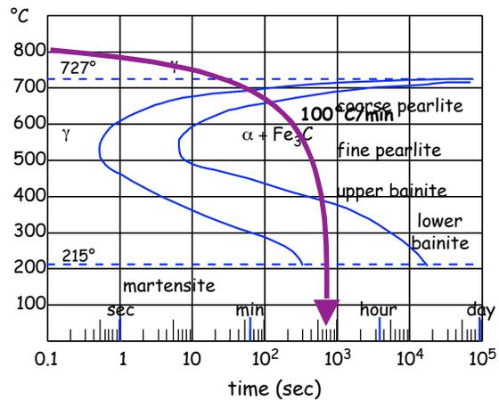
In question (d), note that a linear rate of 100°C / min is dramatically curved on the log scale used here. Although this is only an "approximation" because the cooling treatment is not isothermal, it is reasonable to expect that the final microstructure would be fully pearlitic, and rather coarse.
