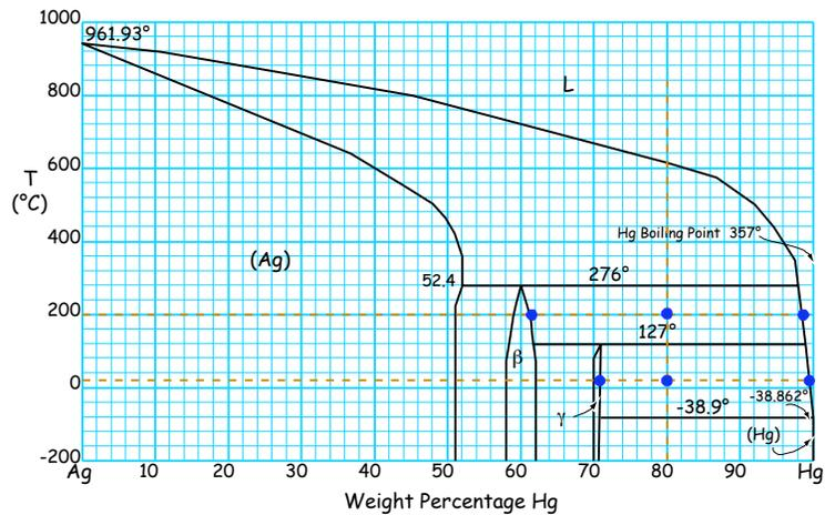
Note that in all cases here, there are no microstructural remnants from higher temperature reactions to influence the products. All are peritectic reactions, which require longer times to reach equilibrium, but time is not a factor here since we are working from an equilibrium phase diagram.
