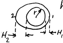
$$h = r v_\theta = \text{CONSTANT. } r_1 v_{\theta_1} = r_2 v_{\theta_2}$$
