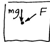
(a) CONSTRAINTS:  $r = \text{CONSTANT}$  HENCE  $\dot{r} = \ddot{r} = 0$ . SLIDING FRICTION IMPLIES  $F = \mu N$  WHERE  $N$  IS NORMAL FORCE.  $\vec{F} = -\frac{\mu N \vec{v}}{\sqrt{v_\theta^2 + v_z^2}}$
