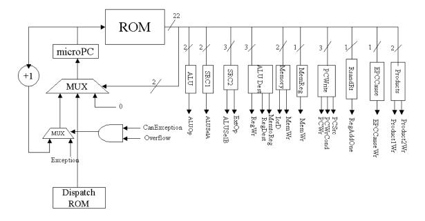
2 points were given for drawing a decent microcontroller for the old datapath. 1 point was given if the branching (exception) mechanism was implemented with a mux. Another point was given for showing some new control signals (EPCWrite is the most notable).
