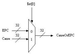
2) Expand MemtoReg mux to take in the CauseOrEPC.
