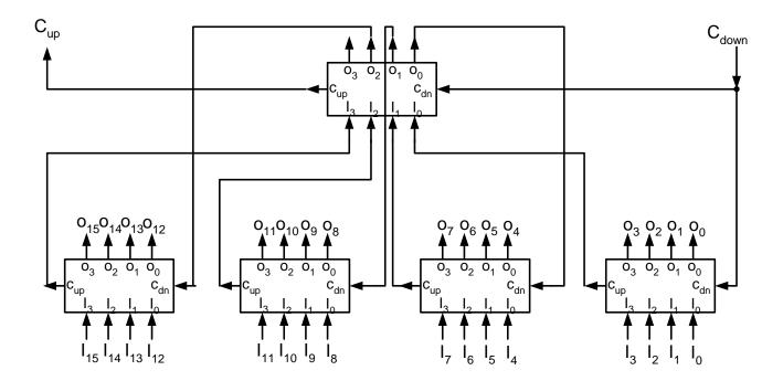
The critical path is from  $I_0$  up through the central logic and back through the  $C_{down}$  of the last stage to  $O_{14}$  or  $O_{15}$ .
