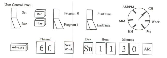
The user console works in the following way. SET/RUN, Program 0/Program 1, and StartTime/EndTime are toggle switches. With the switch's top pushed in, the top signal is indicated (e.g., Set, Program), StartTime). When the bottom is pushed in, the lower signal is indicated (e.g., Run, Program1, EndTime). Record and Play are indicated by push buttons: when first pressed, the indicated signal is asserted. When pressed a second time, the signal is unasserted.
