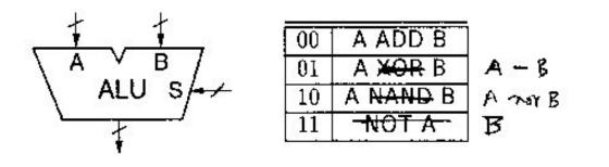
Instructions are in the form of: OP ADDR with 2 bits for the OP field and 6 bits for the ADDR field.
