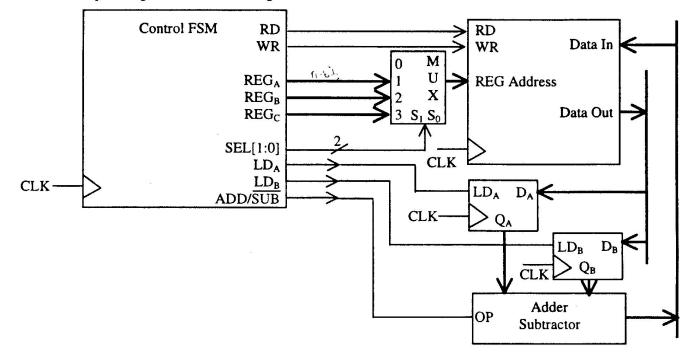
Draw the state diagram fragment below, annotating the transitions with the asserted control signals to implement the read/operate/write sequence:
