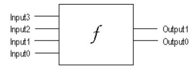
At least one of the inputs is always asserted high. If a give input line has a logic one applied to it, then the output signals will encode its indes in binary. For example, if input Input2 is asserted, then the output reads Output1 = 1, Output0 = 0. If two or more inputs are at a logic one, the output will be set according to which input has the highest index (Input3 > Input2 > Input1 > Input0).
