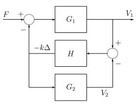
(c) Find the transfer function from F to  $V_1$ .
