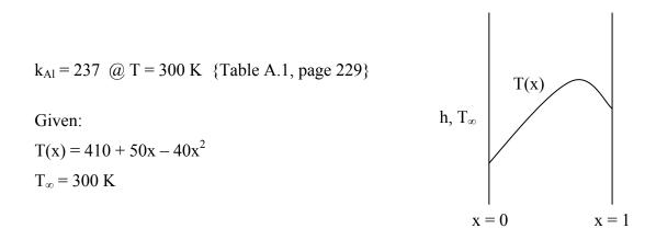
Use temperature distribution to find T(x = 0) = 410 K, thus heat transfer is to the left. At the left boundary the heat rate balance is:
