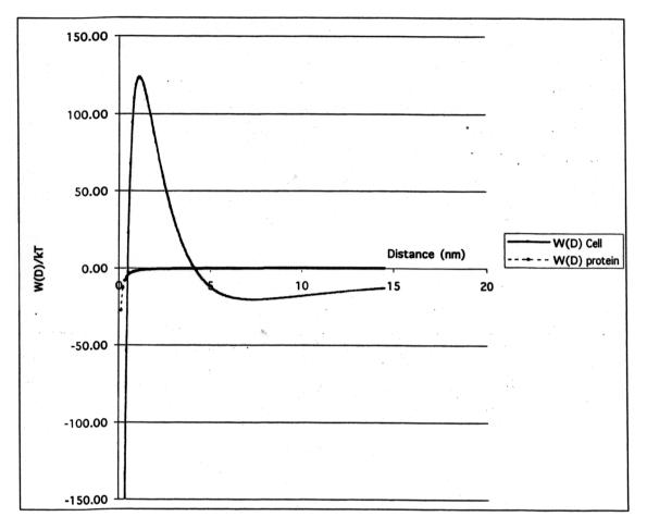
The curves were generated using the following parameters: polymer surface potential of -8 mV; surface potential of -10 mV for the cell; surface potential of -10 mV for the protein; a 1:1 electrolyte with a concentration of 0.2M and a Debye length ( $\kappa^{-1}$ ) of 1.48 nm; at body temperature (37 °C). The diameter of the cell was 10  $\mu$ M and the protein 30 nm.
