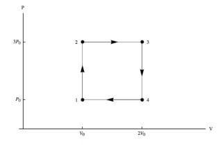
**a.** We can figure out when heat is flowing in by using the First Law of Thermodynamics in the form  $Q_{\rm in} = \Delta E + W$ . If  $Q_{\rm in}$  is positive during some part of the cycle, then that part of the cycle contributes to  $Q_{\rm H}$ . From this rule we see that heat flows in during the processes  $1 \rightarrow 2$  and  $2 \rightarrow 3$ .
