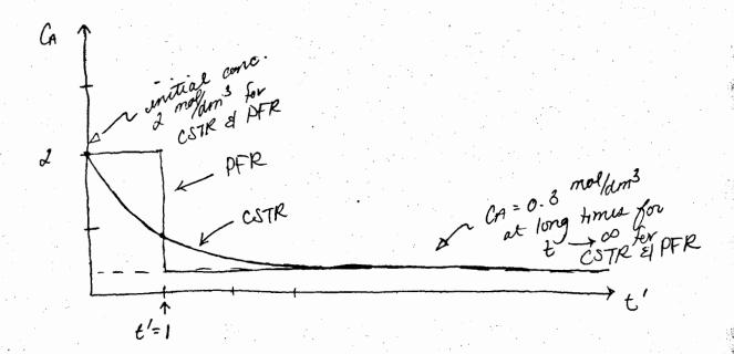
d. On the same plot as part c, sketch the concentration exiting a PFR as a function of t'. You may assume the PFR has the same residence time and the same initial and inlet concentrations of dye. Again, clearly label the concentration at t' = 0 and its value at very long times. Also label on the plot for the PFR where t'= 1.
