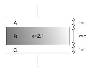
Figure 1: Capacitor with dielectric halfway between plates
