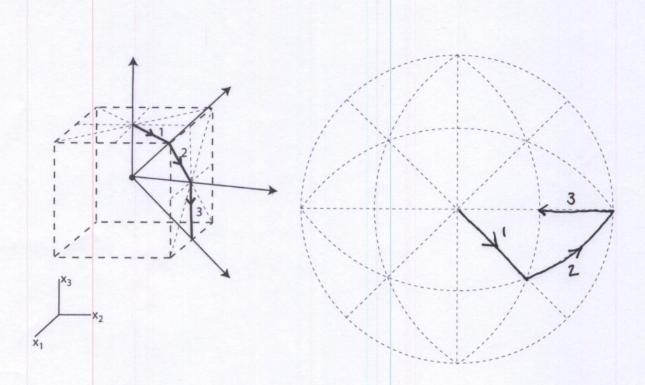
(2) [5 points] A portion of a simple cubic lattice is plotted below. Use this plot to sketch the plane that intersects the  $x_1$  axis at 2, the  $x_2$  axis at 1 and the  $x_3$  axis at 1. Give the Miller indices of the plane that you sketched.
