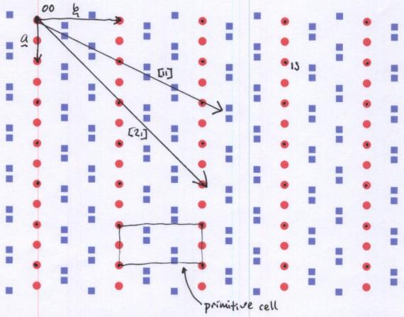
(32) (3) A portion of a two dimensional crystal is shown above. The circles represent one type of atom, the squares another.
