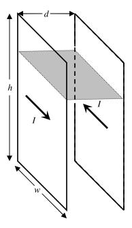
a) **Derive** the magnetic field between the two planes in terms of the current <u>density</u>, *i*.
