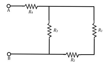
b) If the terminals A and B are connected to a battery with voltage V, find the power dissipation for each of the four resistors. Express your answers in terms of V and R.
