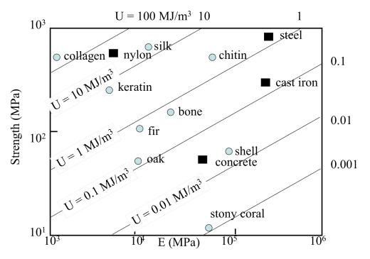
a) Oak and fir can't have the same E, because the stress measured in fir is higher when measured in tension. True or false given the following data? Fir stress = 70 MPa; strain = 0.007; Oak stress = 40 MPa; strain = 0.004. Assume Hookean behavior. Justify your answer by calculating E and comparing directly. (5 points)
