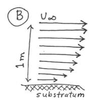
The arrows, which represent velocity vectors, are drawn to the same scale in A and B.
