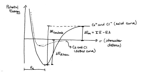
(b) Estimate the dissociation energy of CsCl (in kJ/mol) relative to the separated atoms, use a bond dissociation of  $R_e$ =3.222 Å (1 Å =  $10^{-10}$ m). State any approximations you make.
