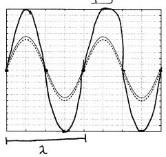
(b) Shown below is a plot of the electric fields of two blue, 400 nm light waves that are  $180^{o}$  ( $\pi$ ) out of phase with each other. On this figure draw the wave that would result from the interference of these two waves.
