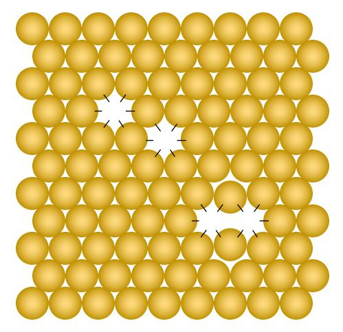
The simple explanation here is that the creation of a single vacancy in the (0002) planes requires the breaking of six bonds. Two isolated vacancies therefore have twelve (12) broken bonds, but a single divacancy has only ten (10) broken bonds. The *energy difference associated with these two (2) bonds* makes the divacancy more favorable because it has a lower energy.
