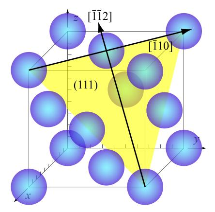
The dot product between **b** and  $\xi$  is zero, so they are perpendicular, meaning that the dislocation is, by definition, a pure **edge dislocation**. The directions of both **b** and  $\xi$  are illustrated on the drawing above.
