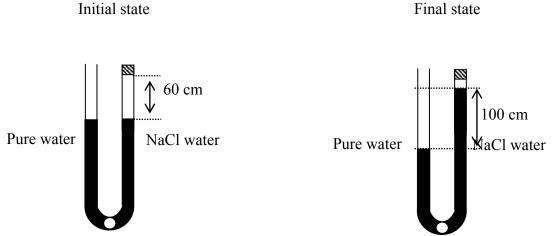
Data: Initial pressure both outside and inside the tube is 1 atm.  $T = \overline{298}$  K. The tube is sealed on the right side, but is open on the left. The semipermeable barrier at the bottom is fixed in place and allows water, but not ions to pass. A  $\Delta P$  of 1 atm can raise a column of water 1 m.
