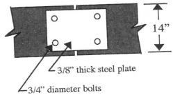
AS THE WOOD SHRINKS, THE BOLTS MAY NOT MOVE RECATIVE TO EACH OTHER SUFFICIENTY TO RELIEVE THE STRESS AND THE WOOD MAY SPLIT ALONG THE GRAINS AT BOLTS.
