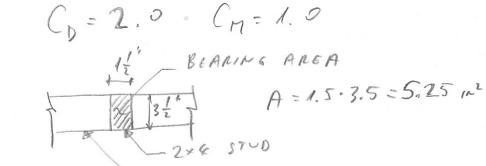
REARING STRESS PERPERDICULAR TO GRAIN:
