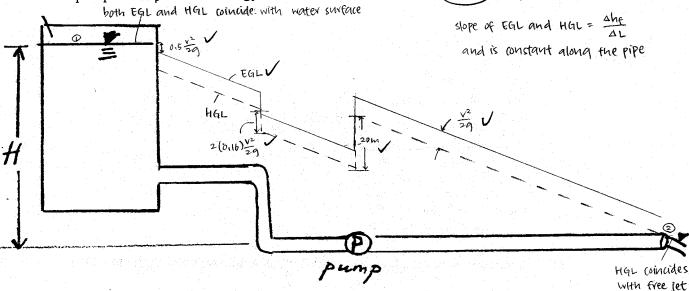
2a.) Sketch the energy grade lines and hydraulic grade lines for the pipe system. Point out the important features, especially if you can't draw very well. (5pts)
