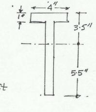
2. Facting downward Top in compression Bottom in tension  $T_{top} = 6000 = \frac{25 \cdot 2F \times 3 \cdot 5}{97} \Rightarrow F = 6599$  lb  $T_{bot} = 3000 = \frac{25 \cdot 2F \times 5 \cdot 5}{97} \Rightarrow F = 2100$  lb  $\vdots T_{bot}$  governs  $\Rightarrow F = 2100$  lb F = 2100 lb F =
